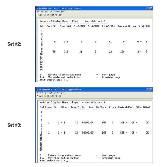
Second and third columns show groups and phase ownership. Next columns show module serial number and software version. Last columns show the alarm code and the status of each module port:
