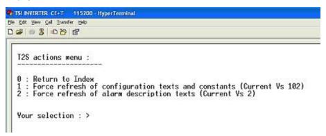
By default the T2S detects automatically when more recent TSI modules are inserted in the system. It updates accordingly the internal description of parameters and messages.
