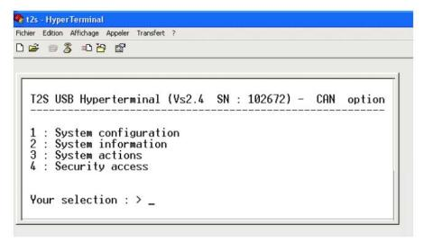
The software version of the T2S as well as its serial number is displayed on this screen.
