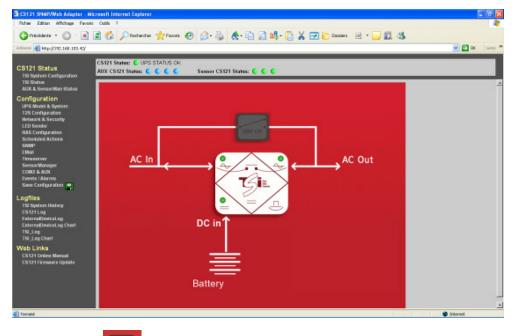
On above screen, the "MBP" box **I** is greyed because there is no MBP present on this system or because the text configuration in the T2S file is not correct (see line 901 in section 7.6, page 57).
