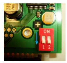
Please note that, in "Normal position" Dipswitch "1" is on the "ON" position and Dipswitch "2" is on "OFF" position. These are the positions when TCP IP in mounted on CanDis in the CE+T Factory.
