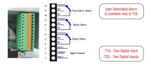
All alarms are qualified in Minor alarm except the one configurable by T2S. These configurable alarms are identified by the ID601 to 900. Refer to list of factory settings (see 6.9.5, page 26)
