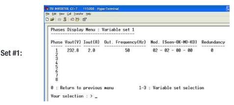
The phases that are recognized by the system are listed here-below and show 3 sets of parameters.
