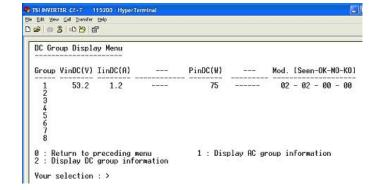
The last column displays a string of digits showing the list of modules recognized by the system in this particular group:
