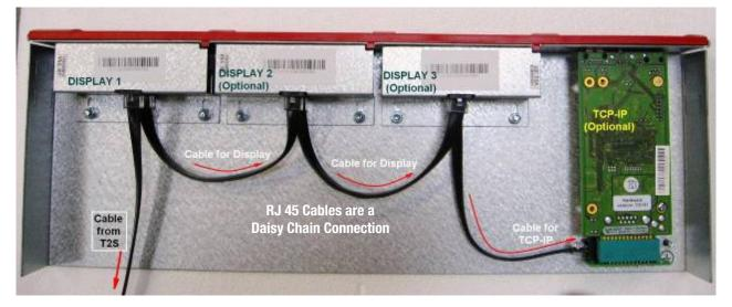
When there are more than one displays in the CanDis shelf, connect the provided set of cables with the device between the free terminal on display 1 to display 2 and the same for the third display.
